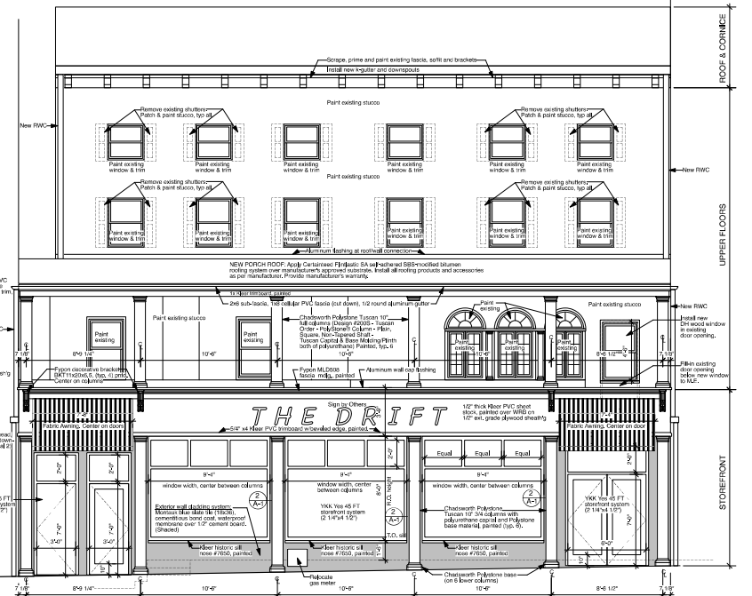
BRIDGE STREET FAÇADE SCALE: 1/4"=1'-0"
